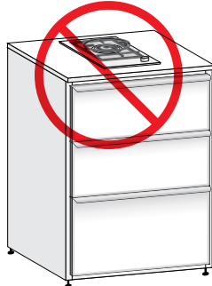
671 Drawer Unit Wok Burner is NOT installed
